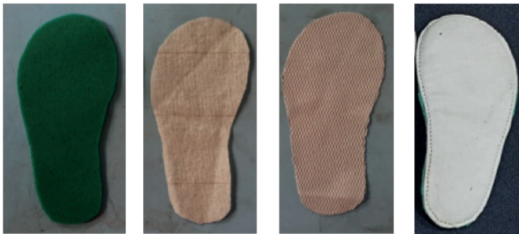
Figure 1. Representative images on the components of foot-bed materials used for the preparation of a complete foot-bed. The synthetic foot-bed materials composed of a fabric, lining and foam materials and the leather-based foot-bed material composed of a leather material of bovidae origin
