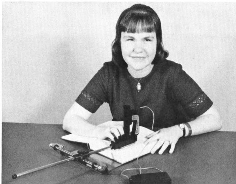
Figure 5a. Miss Bonnie Reinicke is shown using the Visotactor B and Colineator to read a book. She has used this equipment in her home since September 1964.
