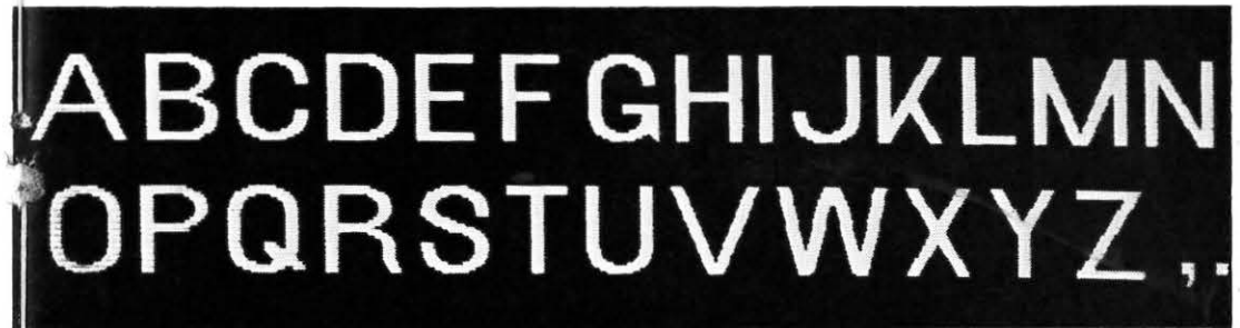
Figure 11. Video image of intermediate stage of Vidifont character. Curves are still flat-sided.
