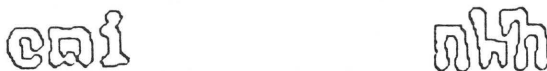
Figure 11. The smearing of nearby lines by convolution. Left: “emi” – for strokes within a character. Right: “nWh” – between two characters.
